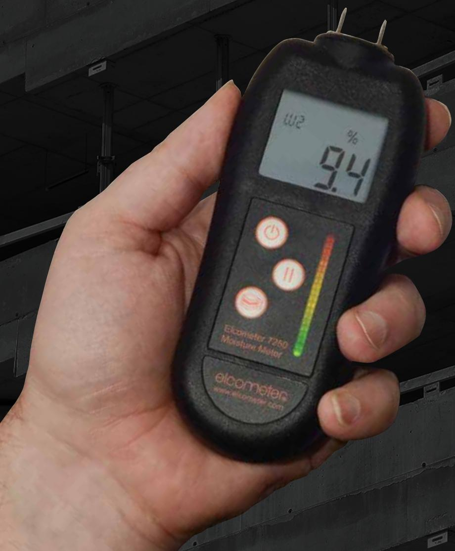
Accurately assess moisture levels in wood, plaster, and concrete prior to coating to prevent structural damage.
